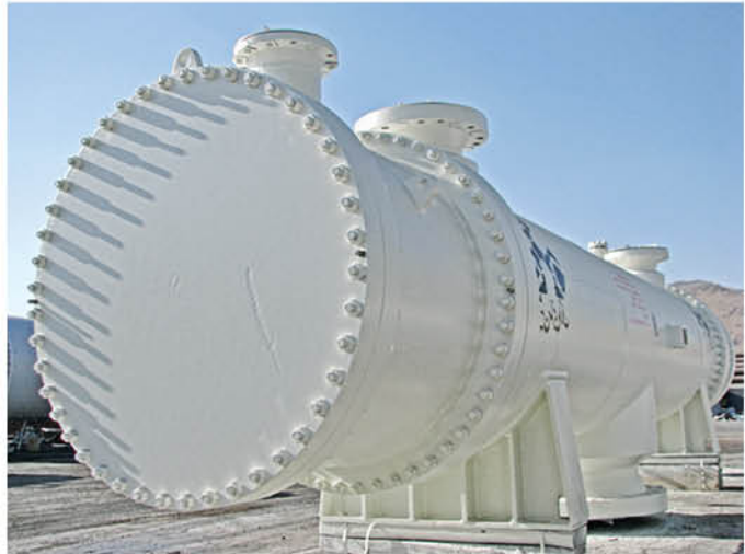
South Pars phase 14, titanium heat exchanger
